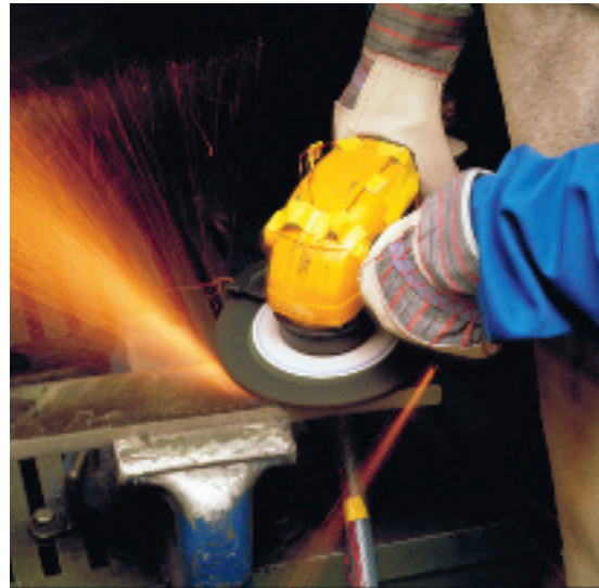
Grinding wheel imbalance is one of the main sources of vibration.
