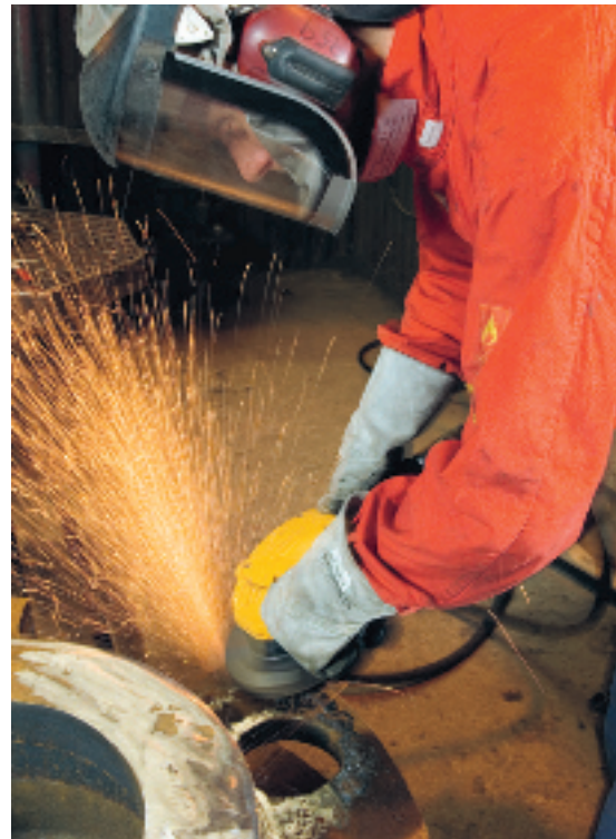
Modern turbine grinders can preferably be run on non-lubricated air.
