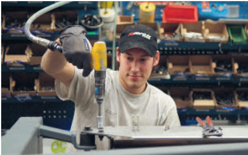
The selection of handle type can have an adverse effect on posture.
