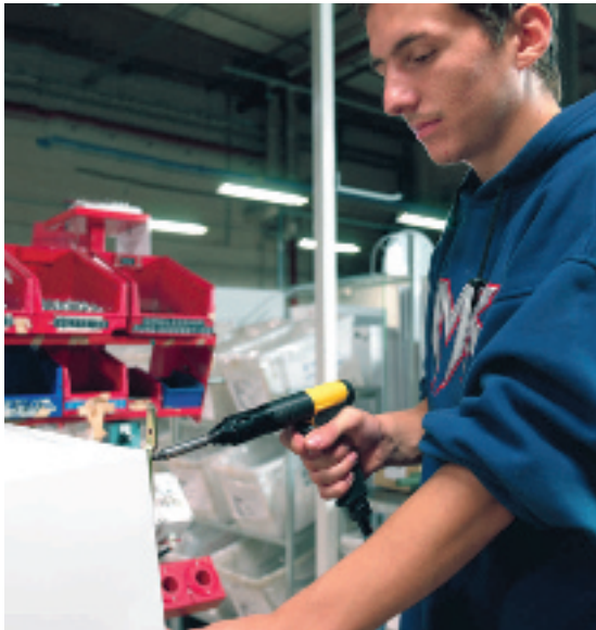
The textured viscoelastic grip serves to reduce contact forces.
