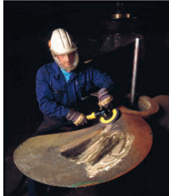
Hand-held grinding is often more flexible than using numerically controlled machines.
