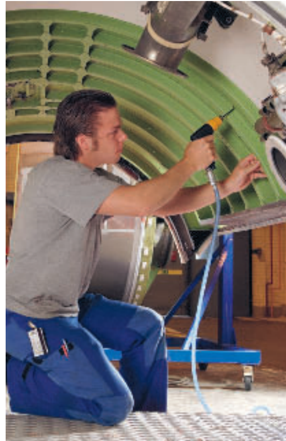
A small, modern drill must be designed to give the operator a choice between high and low grip.
