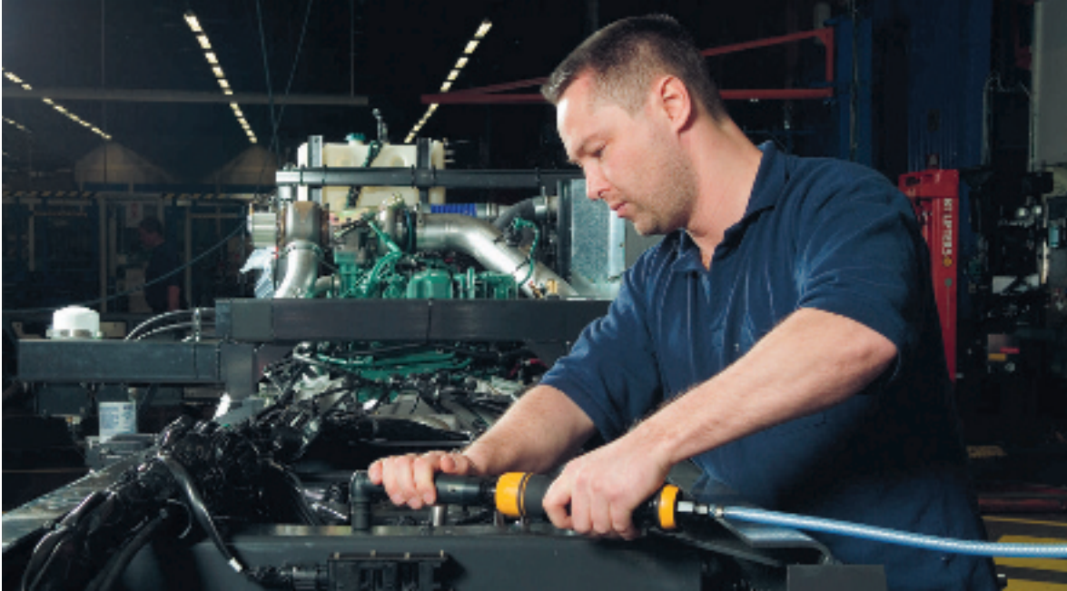
High motor power and fast clutches are important to reduce the shock reaction from angle nutrunners.
