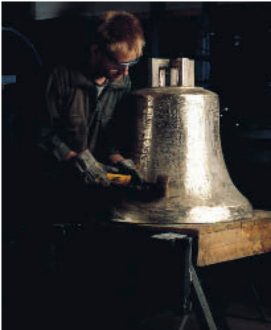
Hand-held grinding is often more flexible than using numerically controlled machines.
