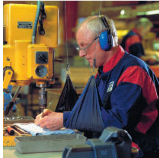
Arm slings compensate for the weight of the arms, and reduce tension in the shoulder-neck area.
